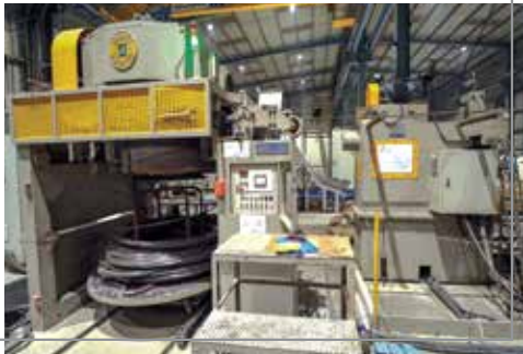
Wire Drawing Machines Dia: 8mm-32mm
